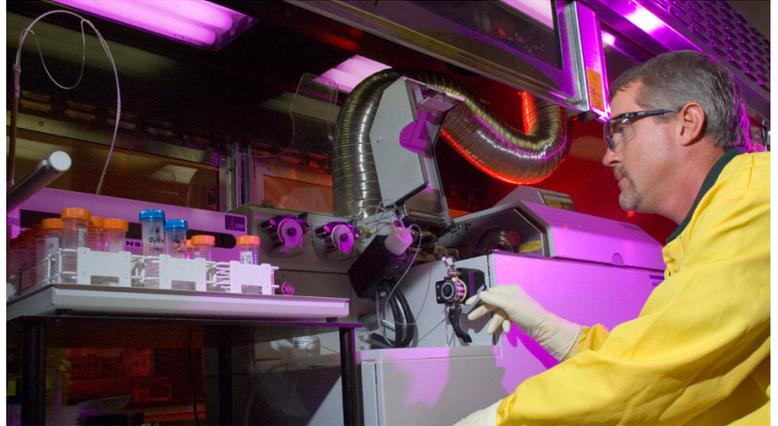
*A lab employee performs technical oversight of an Inductively Coupled Plasma-Mass Spectrometer.*
