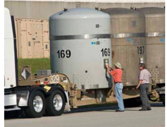
Preparing a shipment of TRU waste in TRUPACT IIs for shipment to WIPP.
