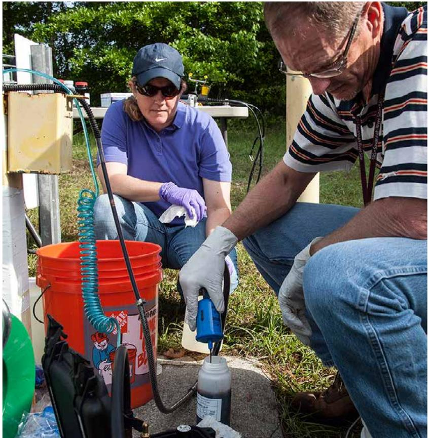
*Geologists Maggie Millings (left), and Mark Amidon, both with the Savannah River National Laboratory Environmental Restoration Technology Section, conduct tests used to monitor groundwater retrieved from wells near F Area at the Savannah River Site.*
