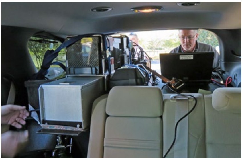
Radiological Assistance Program 3 team member and SRNS employee Mike Conaway completes software connections for mobile detection equipment. RAP 3 personnel conduct real-time monitoring of gamma and neutron radiation detection equipment as it is deployed in the field, often at major public events.
