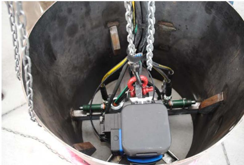
The diagram shows the innovative concept for the canister double-stack project. Canister positions are modified using a specialized cutting tool to accommodate two canisters per existing slot.
