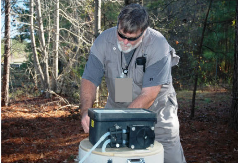
An Automated Water Sampler is programmed at an Industrial Wastewater Outfall
