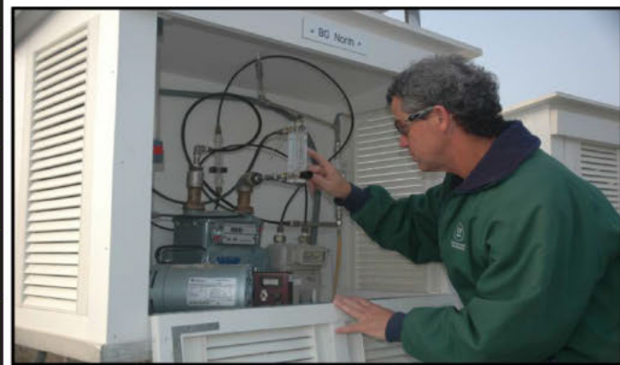
Technician Reads Air Flow at Air Station
