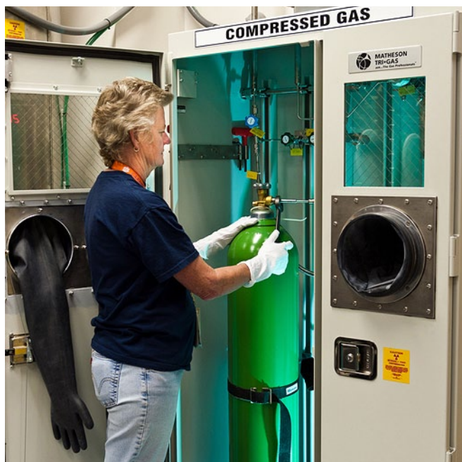
Operator Cindy Sizemore installs a tank to be filled with helium-3, a byproduct of the tritium manufacturing process.
