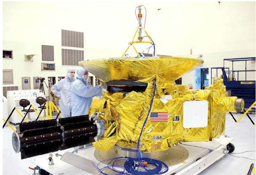
*The New Horizons space probe while in construction. The black, finned extension on the left side of the picture is the RTG.*
