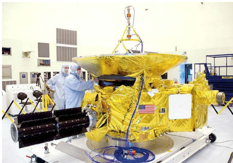
The New Horizons space probe while in construction. The black, finned extension on the left side of the picture is the RTG.
