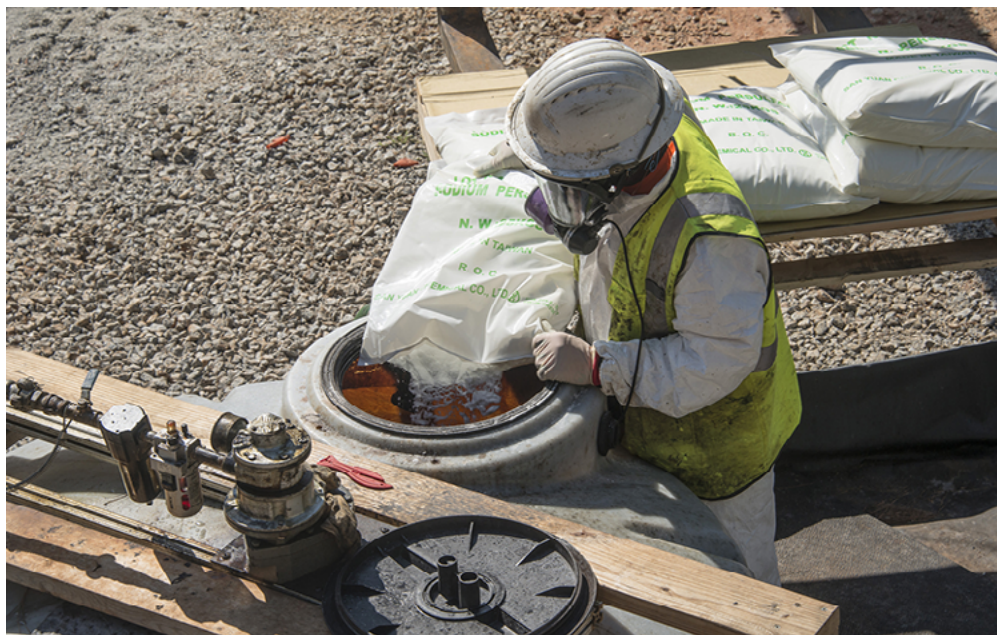
Savannah River Nuclear Solutions is using oxidants to neutralize solvents found in groundwater beneath the Savannah River Site in a field-scale test. The oxidants destroy the waste solvents, producing non-toxic byproducts.
