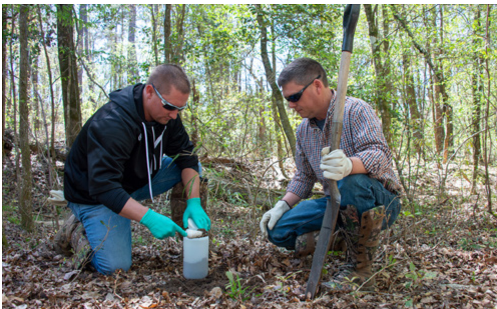
Environmental Monitoring Sample Technicians collect soil samples at an onsite sampling location at the Savannah River Site for radionuclide analysis.
