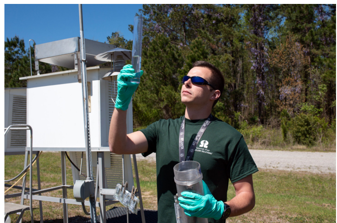
Savannah River Nuclear Solutions Environmental Monitoring Specialist Jesse Baxley reads a rain gauge. Rainwater is one of the SRNS Environmental Monitoring Program's collection media used to ensure SRS operations pose no risk to the surrounding population.
