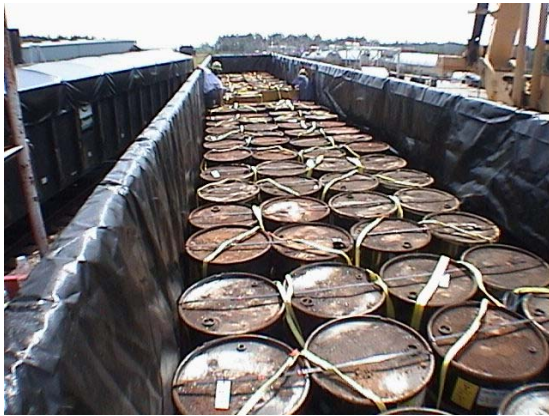
Campaign 1 – 3,270 55-gal drums to UT FY03 Open-top gondola cars w/ "Superload" wrappers as container
