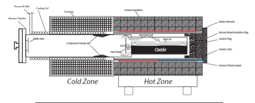
Vacuum Salt Distillation removes corrosive chloride salts from DE3013 oxides. Salts are vaporized and condensed, resulting in clean oxide product and salt waste.
