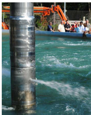
Installing the pump into the test stand
