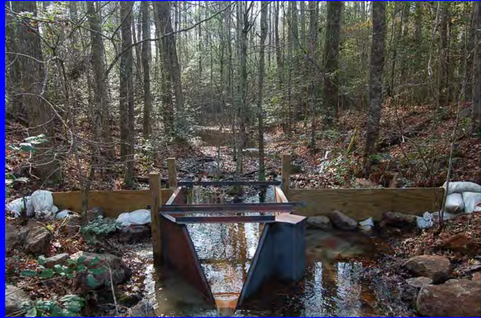
This flume measures storm flow and serves as a sample point for water chemistry samples.
