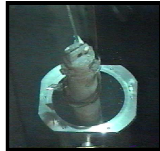
Fuel can loading into Oversize Can
