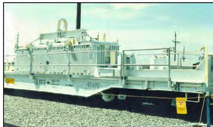
UNF being sent to H Canyon via 70 Ton Cask
