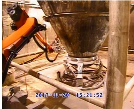
Robotic welding of cap to evaporator vessel
