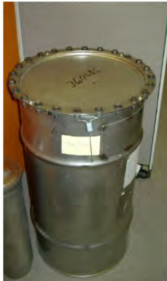
Type B - 9975 Plutonium Shipping container (~400 pounds)
