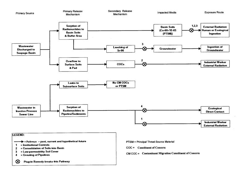
Post-Remedial Action Conceptual Site Model For L-Area Reactor Seepage Basin With Plug-In Rod
