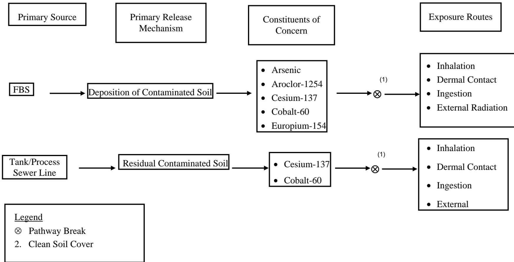
Figure A-1 Conceptual Site Model for FBSB OU with Selected Remedy Applied
