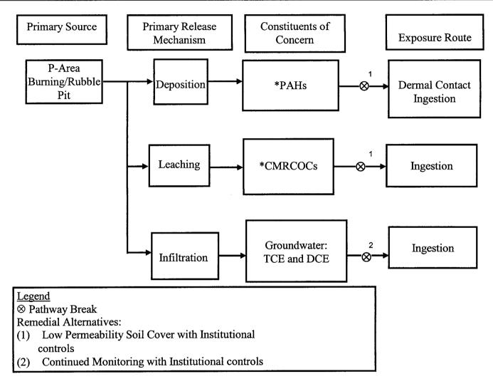
Figure E-1. Conceptual Site Model for the PBRP with Remedy Applied
