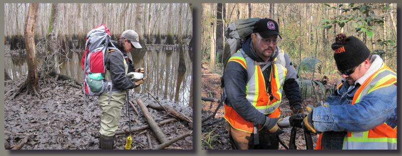
Above left: A member of the survey crew uses an LaBr gamma detector on a sample of vegetation. Above right: A handheld computer is used to record the results of the LaBr survey.
