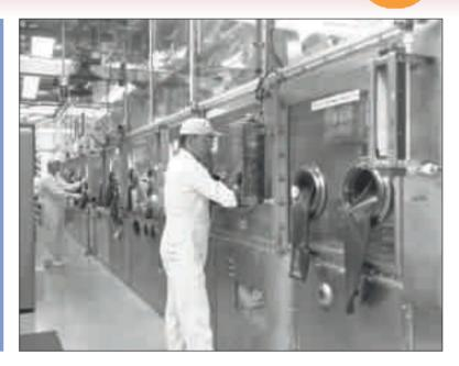
Upper Right: Workers Using Gloveboxes to Isolate Hazardous Materials at SRS.
