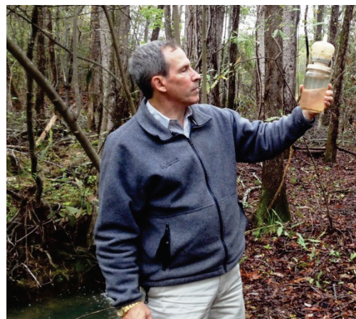
Figure 4-9 Visual Assessment of an Industrial Stormwater Outfall Sample
