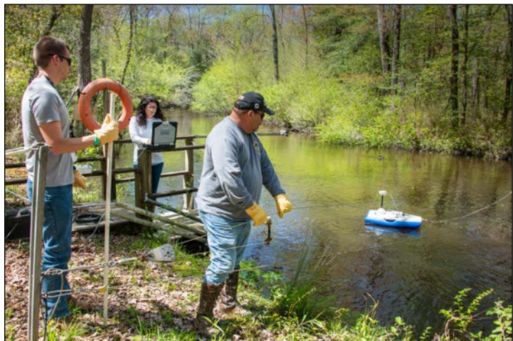
Field Personnel Measure Stream Flow Using River Surveyor
