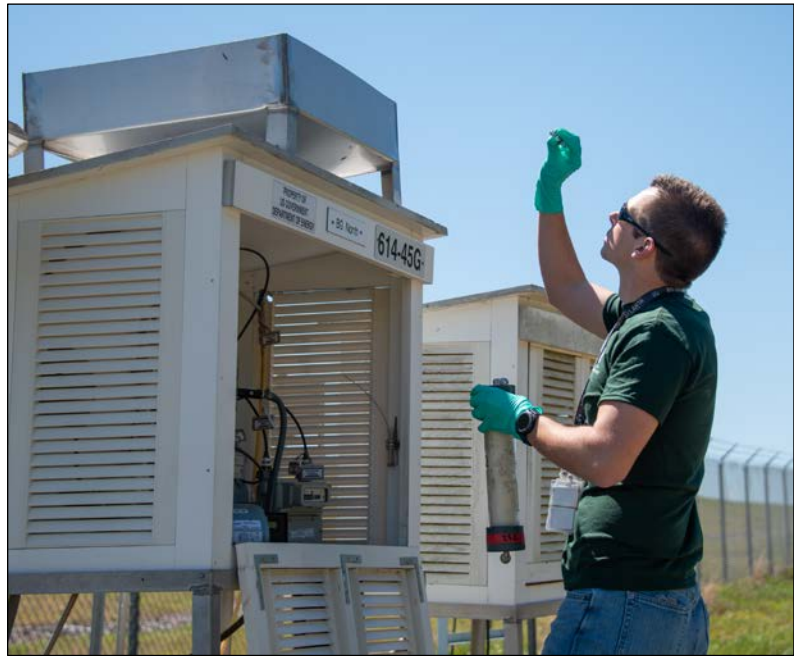
Technician Verifying Equipment Readings at Air Monitoring Station
