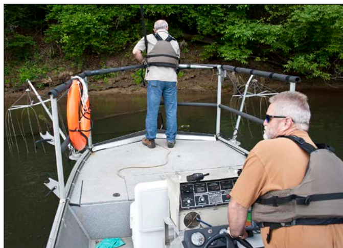
SRS Samples Fish from the Savannah River Using Electrofishing Methods. Radionuclide Concentrations in Fish Harvested from the Steel Creek Mouth are Used in the Representative Person Dose Calculations.
