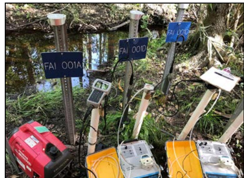
Checking a Passive Soil Vapor Extraction Well (top photo) and Sampling Equipment (lower photo)
