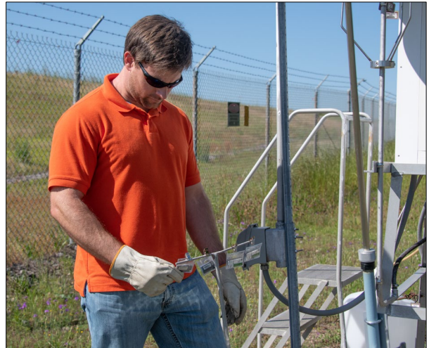
SRS Measures Environmental Gamma Exposure Rates with OSLDs Placed Across the Site for Three Months. The Technology Replaced Thermoluminescent Dosimeters.
