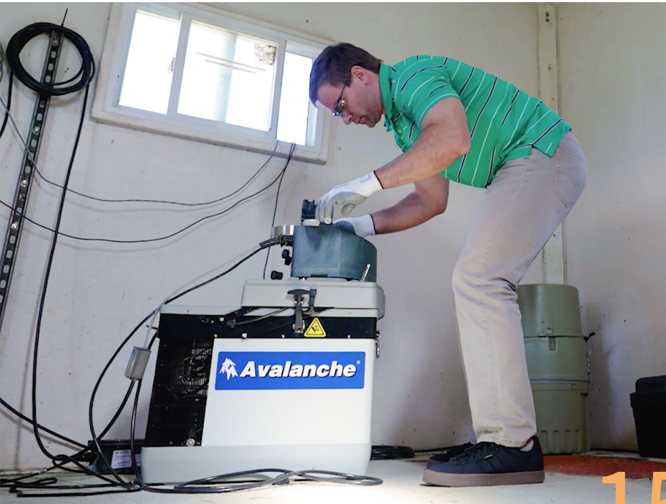
The refrigerated sampler allows Savannah River Site scientists to control and preserve samples remotely, saving time in the field and allowing quick response to emergencies, if needed.
