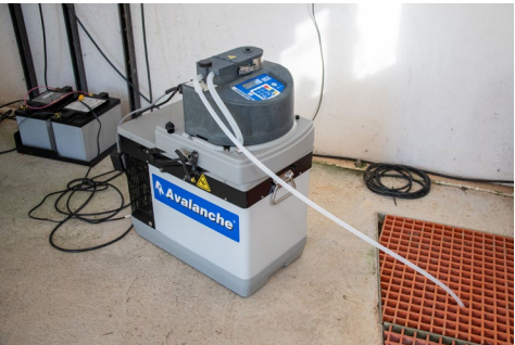
The refrigerated sampler allows Savannah River Site scientists to control and preserve samples remotely, saving time in the field and allowing quick response to emergencies, if needed.
