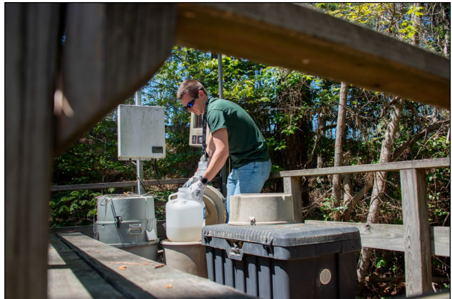
A Jug is Removed from the ISCO Sampler and Taken to the Lab for Analysis.
