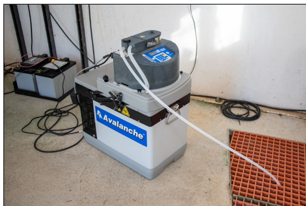
The Portable Refrigerated Sampler Allows for Remote Automation and Calibration Checks.
