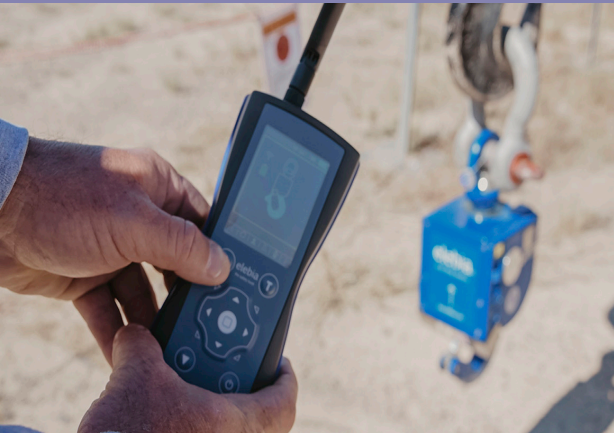
Top: Solid Waste Management personnel inspect a new rigging hook that will aid in placing low-level waste in burial trenches. Above: The hook is controlled remotely, which saves time and enhances worker safety.
