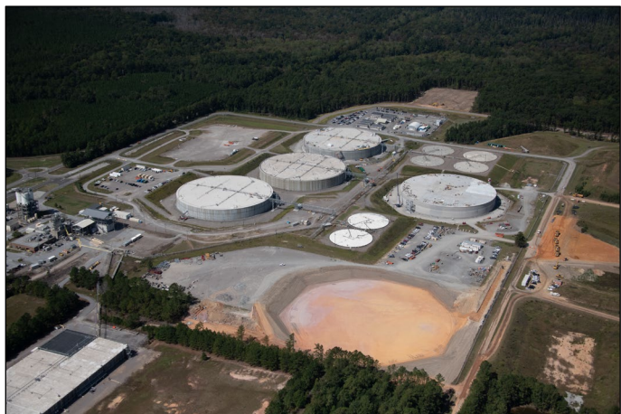
Excavation and Groundwork were Initiated for SDU-11 and SDU-12, the Final Mega-Vaults Planned for Construction.
