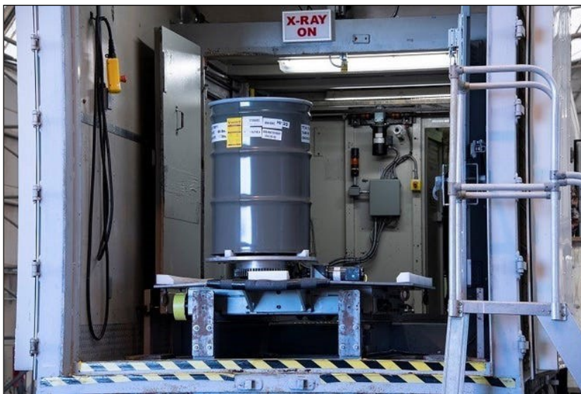
TRU Drum Ready for Characterization in Real-time Radiography Unit
