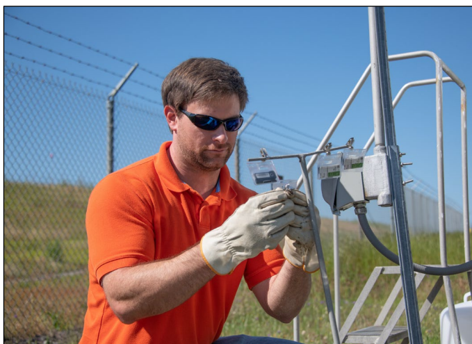
SRS Employee Measures Environmental Gamma Exposure Rates with OSLDs Placed Across the Site.
