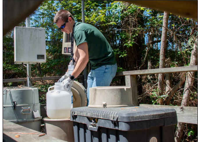
A Teledyne ISCO Sampler Jug is Removed Before Being Taken to the Lab for Analysis.
