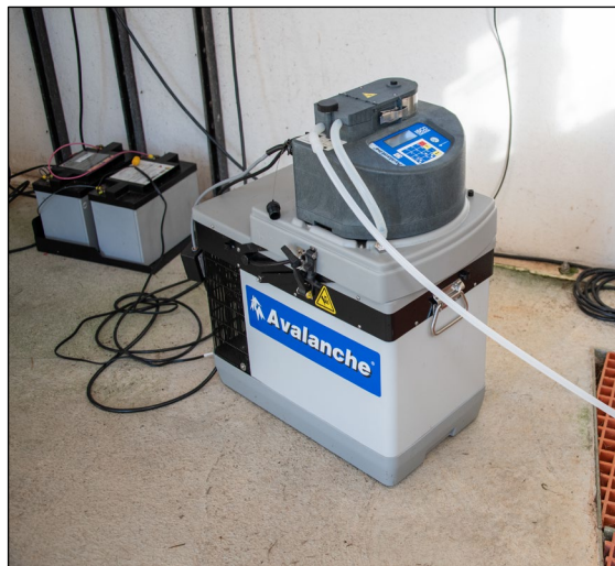
A Refrigerated Sampler Ensures the Preservation of Samples.
