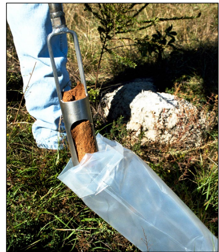
SRS Collects Soil Samples to Test for Radionuclides.
