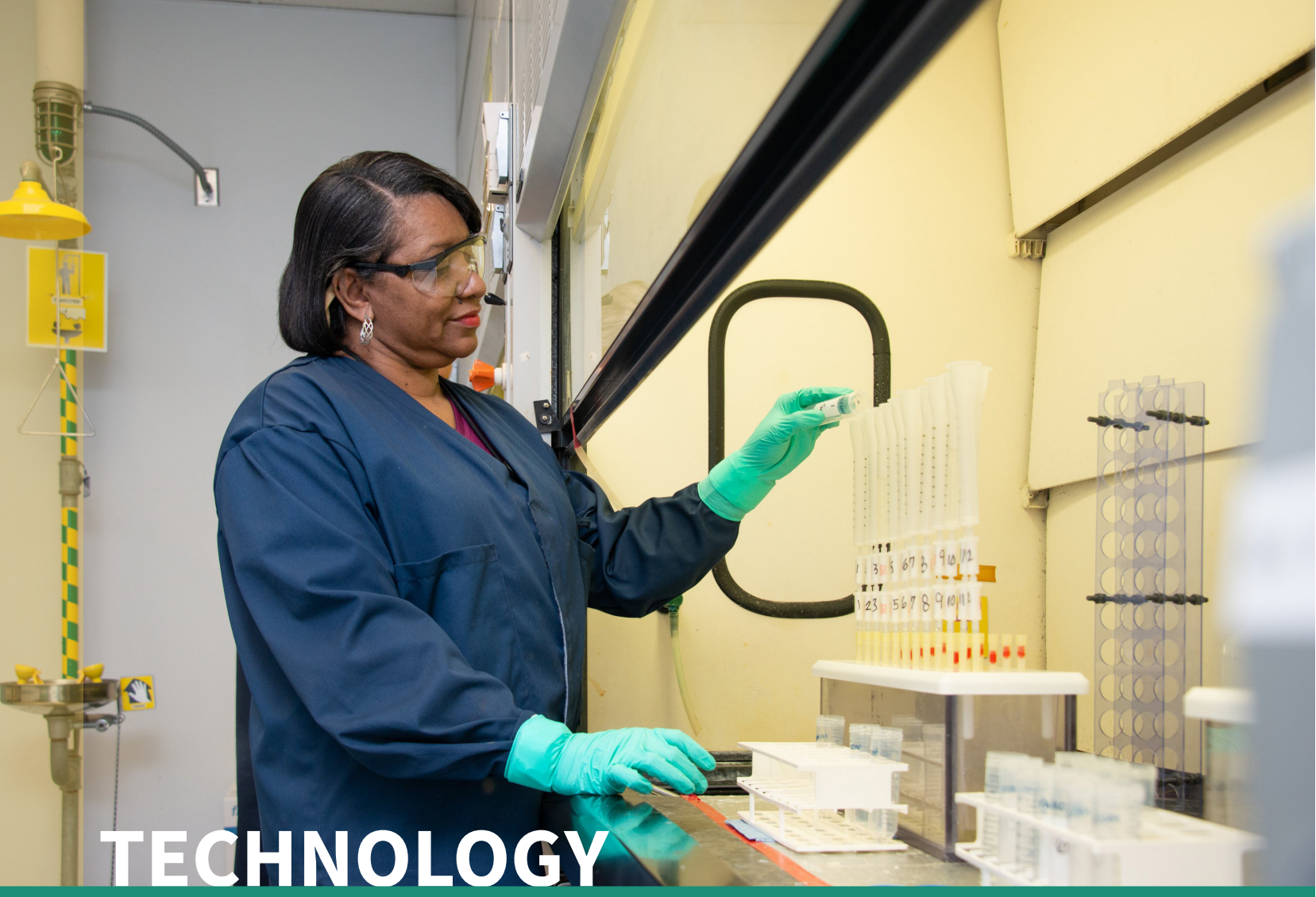
A lab specialist at the Environmental Bioassay Laboratory performs a radiochemistry column separation process.
