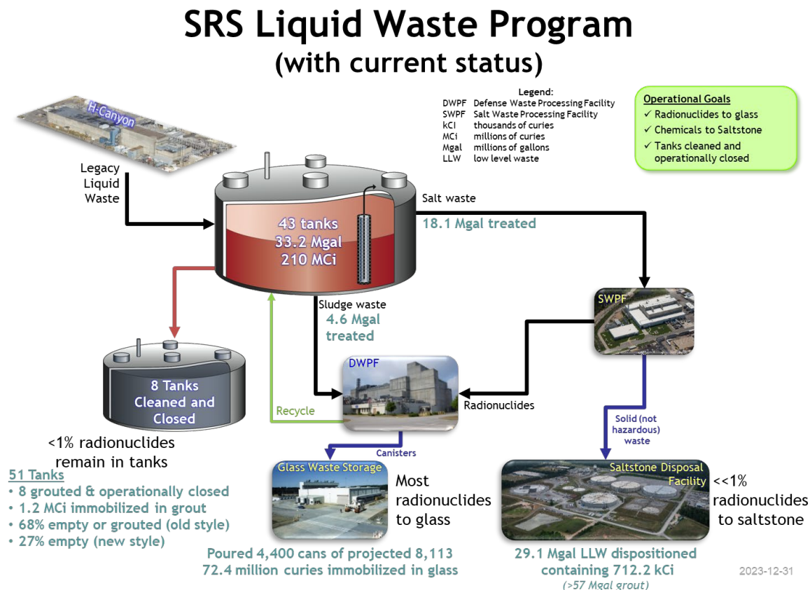
Figure 3-3 Processing and Dispositioning Radioactive Liquid Waste at SRS
