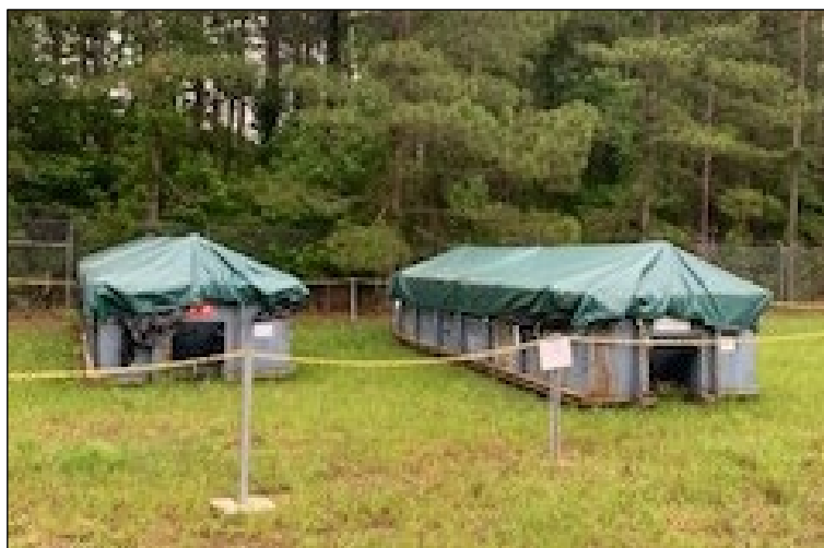
Two Lined 25-Cubic-Yard Roll-off Containers Hold a Mixture of Liquid AFFF and Portland Cement, Which Hardens Into Solid Concrete Blocks.
