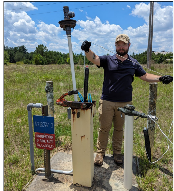
A Sampler Installing a Chain of Passive Diffusion Bags in a Well to Obtain Depth Discrete Samples from Multiple Intervals.
