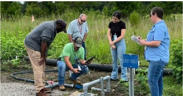
D Area Groundwater Treatability Study project team assesses artesian flow into injection well.
