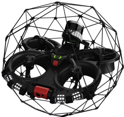
Drones equipped with cameras are used to inspect the cleaning status of waste tanks onsite.
