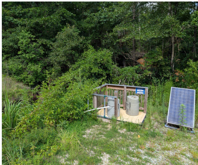
Equipment setup for stream sampling at the new sampling location behind F Area/Shane Shull, SRNS
