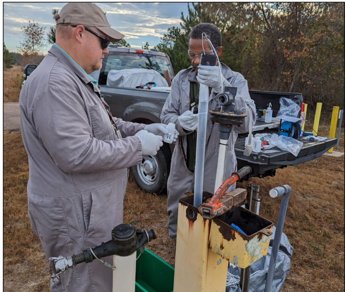
Samplers Collecting PFAS Samples from a PFAS-Free HydraSleeve Bag .
