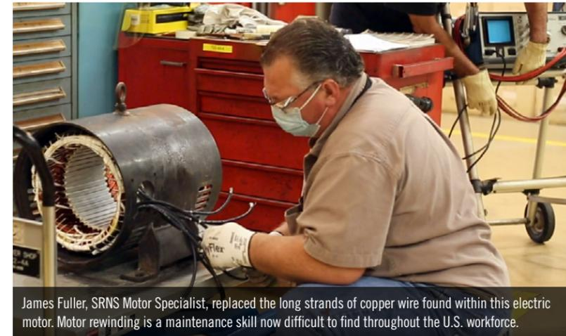
James Fuller, SRNS Motor Specialist, replaced the long strands of copper wire found within this electric motor. Motor rewinding is a maintenance skill now difficult to find throughout the U.S. workforce.
