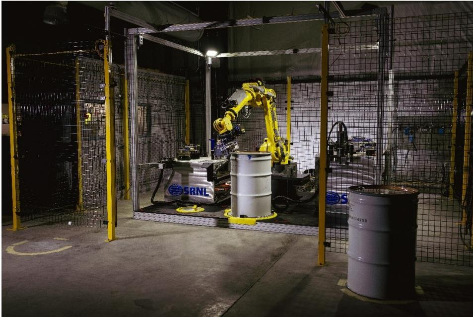
*The Criticality Control Overpack inspection process will use a robotic arm to perform pre-use inspections and security checks after the drum is delivered to the inspection area by an Automated Guided Vehicle.*
