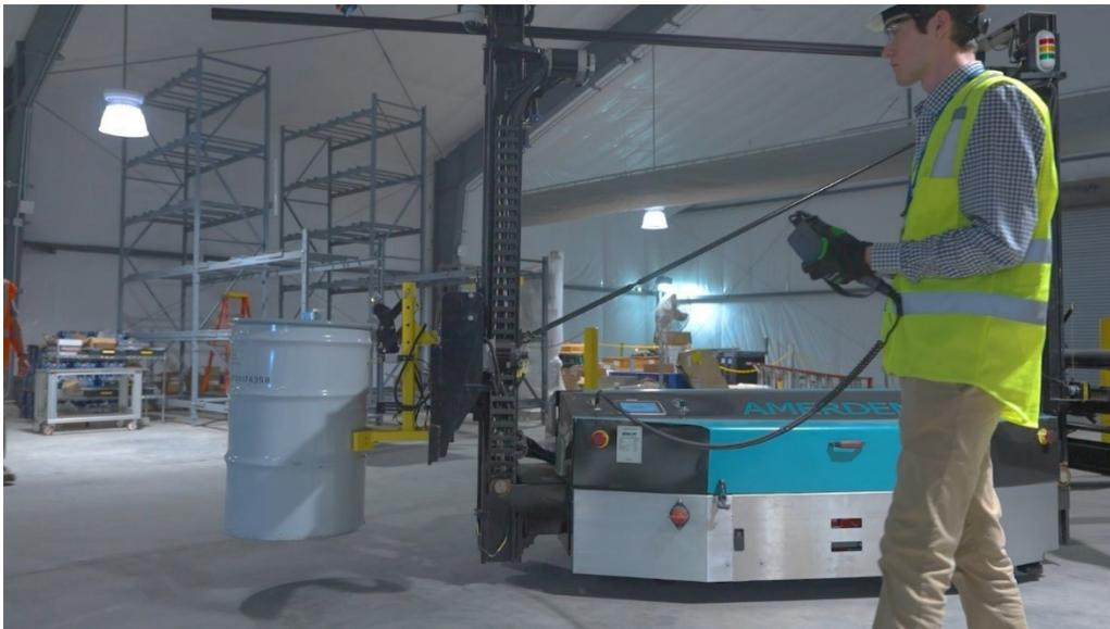
*An Automated Guided Vehicle will be used to deliver shipping containers between staging and shipping inspection locations in a characterization and storage facility at SRS.*
